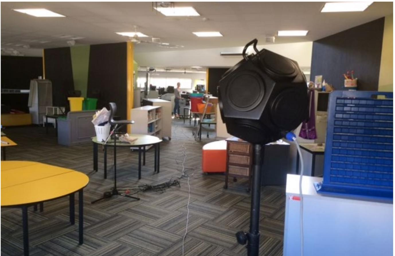
*Signal to noise ratio:* The concept of signal to noise ratio is effectively how loud the source of noise is above the background sound in the space. The larger the difference, the clearer the signal. Guidance from the British Association of Teachers of the Deaf and the America Speech Language Hearing Association suggests that the signal to noise ratio should be at least 15dB, and preferably 20dB in the lower frequency range (125Hz-750Hz).
